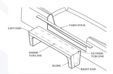
7. Use a tape measure and transfer the shape of the inside of the tub edge to the step. The inside of the tub may be irregular in shape, so measurements for the inside line must be made every 3" from one end of the SureStep Mono Low to the other. Once completed, use your yard stick and marker to connect the markings for the inside line.
